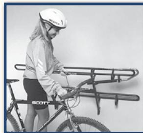
**3.** After lowering the rack, you should place the first bike into the rack's wheel well nearest to the bus. Both bike positions are completely independent of each other, making it easy to load in seconds.
